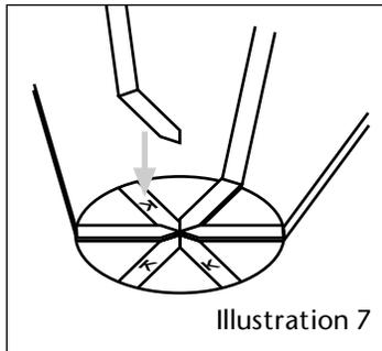
The **Cage Top** is assembled next. Before creating this part, however, another eyebolt must be made following the instructions given earlier. The eyebolt should be a little shorter than the previous one: snip off the ends and leave approx. 1 1/2 loops. Once this eyebolt is complete, punch a hole in the **Cage Top (2c)** part. Push the eyebolt through this hole.
